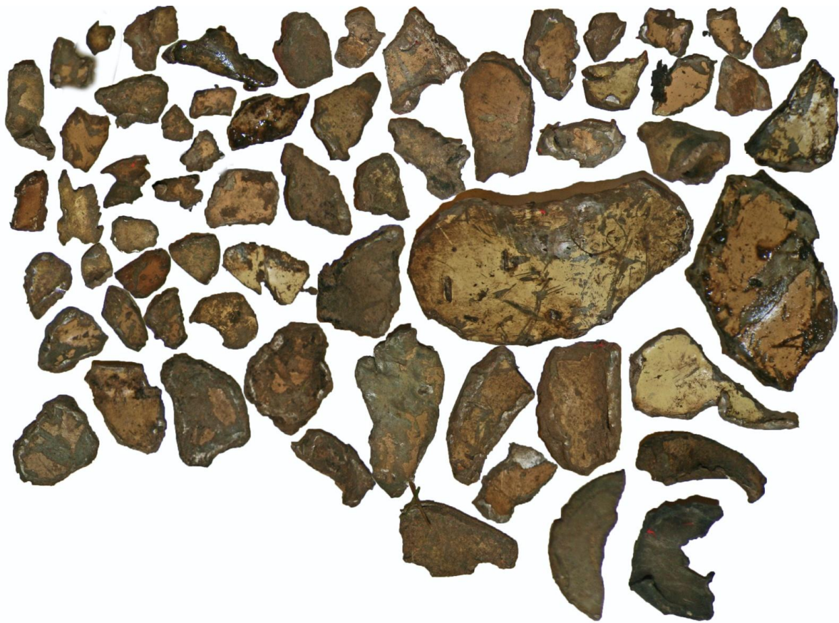
Fig. 33. Pieces collected of the Tu-154M, taken from the ground 100m before the main crash site showing thermal traces.
